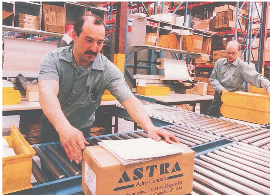
The packing station, at the end of the pick-to-belt system, where shipping cartons are checked prior to weighing, scanning and taping.
